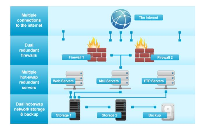
We only use Dell servers in our web hosting platform. Our platform is designed to be highly redundant and all data is stored in network disk arrays.
